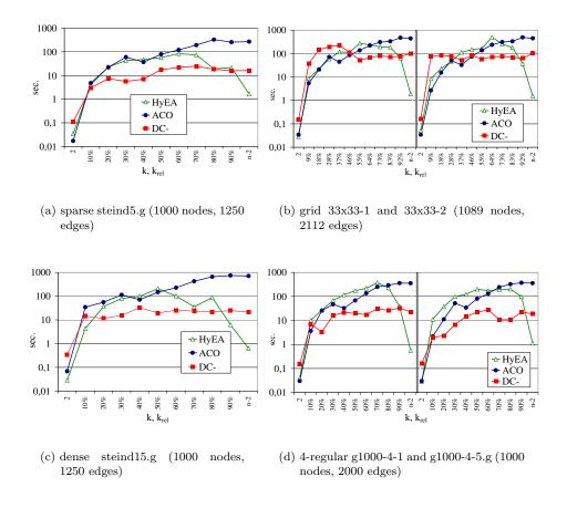
Fig. 6. Running times of DC<sup>-</sup>, HyEA, and ACO (in seconds) for instances of (BB) with  $\sim 1000$  nodes, depending on k. The figures for the grid and regular instances show the times for two different instances of the same type, respectively.
