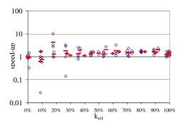
Fig. 4. Speed-up factors for the grid instances of (BB) when gsec-constraints (22) are separated. We have a diamond-shaped datapoint for each instance and  $k_{\rm rel}$  value. This datapoint gives the corresponding speed-up factor achieved by the use of gsec-constraints. The short horizontal bars denote the average speed-up over all instances per  $k_{\rm rel}$ .
